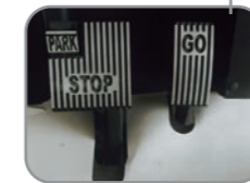
Pedals Integrating acceleration,brake and parking together. Braking distance is adjustable.
